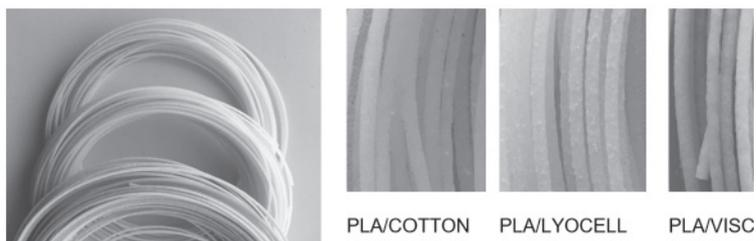
**Fig. 1:** Visual appearance of 3D printable fiber composite filaments.
