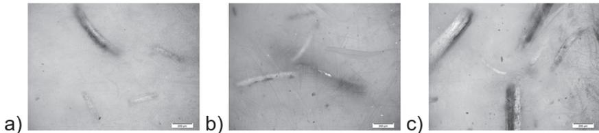
**Fig. 2:** Microscopical images of PCL/PLA/fiber polymeric blends: a) 90/10/0.5, b) 90/10/1 c) 90/10/1.5.
