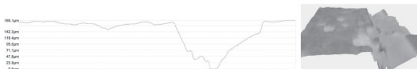
**Fig. 4:** Profile and 3D image of the imprint made by PCL/PLA printing plate.
